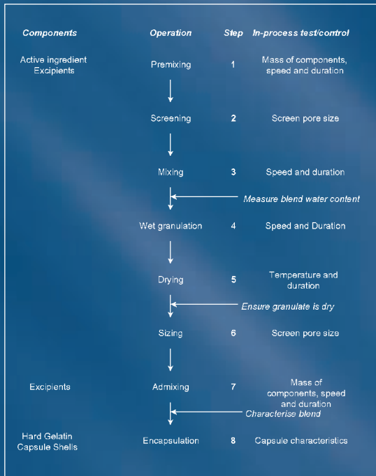
Fig 1. Summary of Typical Manufacturing Process for Hard Gelatin Capsules 1
